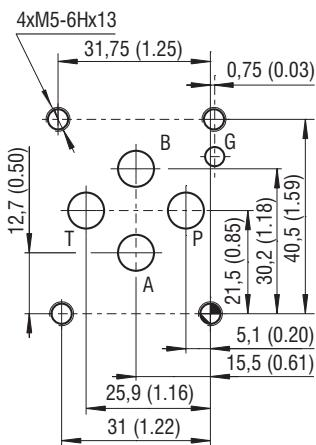
Kanály P, A, B, T - max.  $\varnothing 7,5 \text{ mm}$  (0.29 in)
