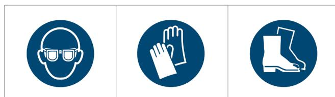
When working with hydraulic fluid, it is recommended to wear safety goggles, protective rubber gloves and sturdy shoes with non-slip soles.
