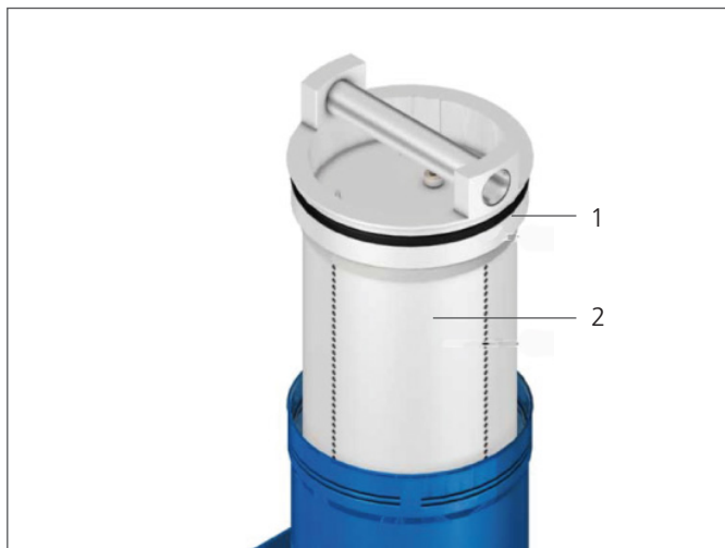
Fig. 20: Installing the filter element
