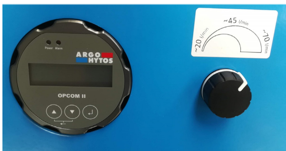
Fig. 12: Front panel with potentiometer for flow adjustment
