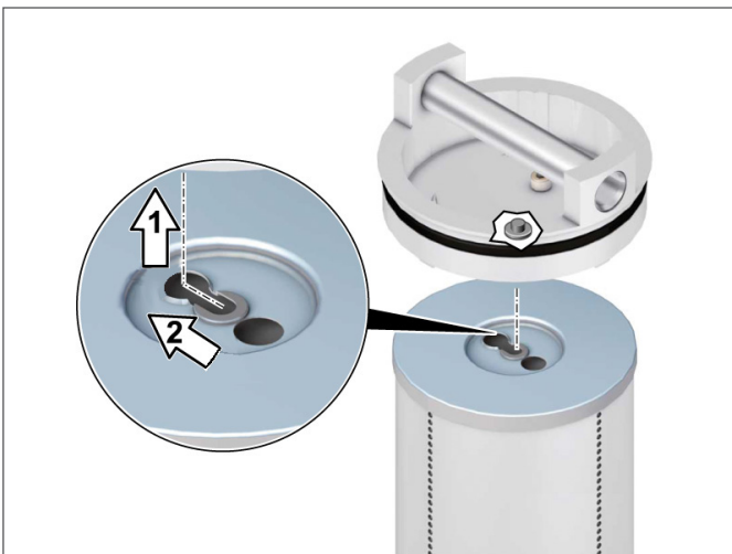
Fig. 19: Attaching the filter element
