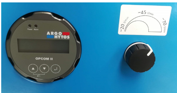
Fig. 12: Front panel with potentiometer for flow adjustment
