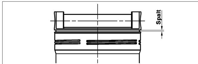
Abb. 36: Spalt am Filterdeckel
