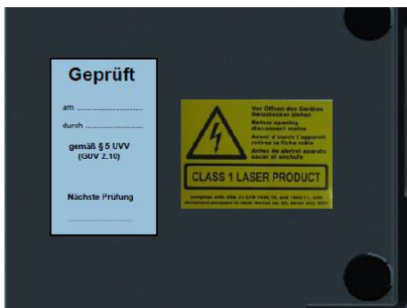
Fig. 1 Bottom of the device with note for the electrical testing and laser protection notice
