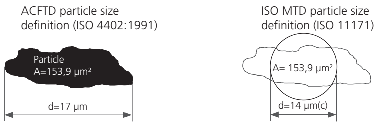
Fig. 31: Particle size definition
