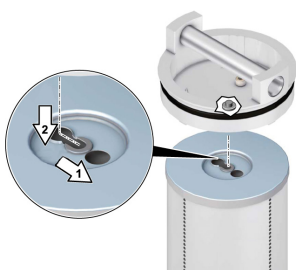
Fig. 5: Removing the filter element from the cover
