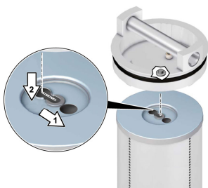
Fig. 5: Removing the filter element from the cover
