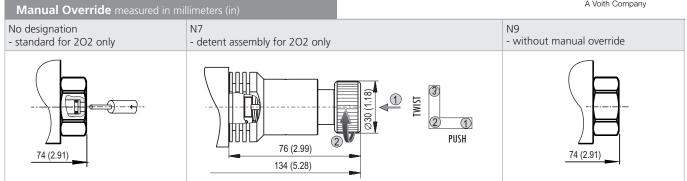
In case of solenoid malfunction or power failure, the valve poppet can be shifted by manual override under the condition that the pressure in the back line does not exceed 25 bar (363 PSI).
