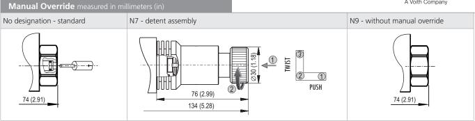
In case of solenoid malfunction or power failure, the valve spool can be shifted by manual override under the condition that the pressure in the back line does not exceed 25 bar (363 PSI).
