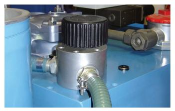
Mounting set attached to the tank
