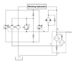
The entire dirt produced in the hydrostatic drive by abrasion is filtered out immediately and is thus not taken in by the pump of the open-loop circuit.
