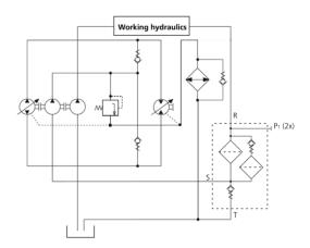
This circuit layout has the advantage that drain oil pressures are comparatively low.
