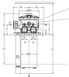
Connection M12 x 1.5 for clogging indicator Return connection A<sub>2</sub> on request
