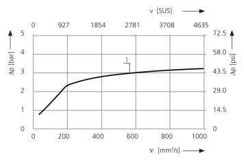
Pressure drop as a function of the **flow volume** at  $v = 35 \text{ mm}^2/\text{s} / 162 \text{ SUS } (00/01 = \text{casing empty})$  without / with hole  $\emptyset 4 \text{ mm} / 0.16 \text{ inch})$
