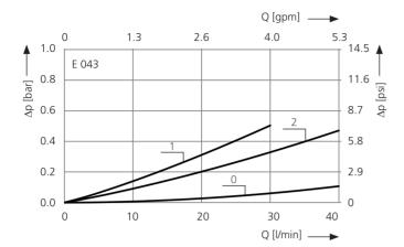
Pressure drop as a function of the **flow volume** at  $v = 35 \text{ mm}^2/\text{s} / 162 \text{ SUS } (0 = \text{casing empty})$
