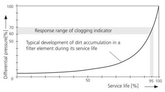
The dirt load collected in a filter element gradually increases during service, which also leads to a higher pressure drop. The resulting differential pressure  $\Delta p$  is monitored by a clogging indicator. Once a preset value is reached, an electrical and / or optical signal is generated.
